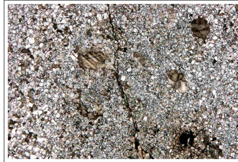
TS W144-13b N35930 PPL x13. Marble; recrystallised sparite with possibly biosparite and possibly remnant crinoid fragments.
