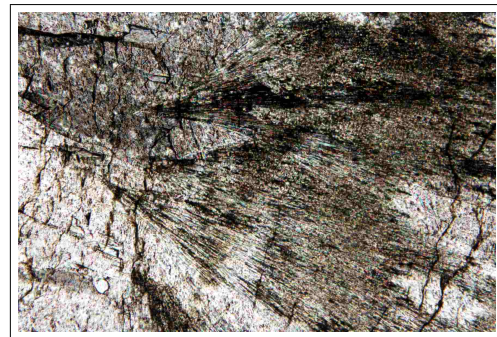
TS W111a XN x50. Powdery needle crystals form islands within the consolidated aragonite and calcite. Calcite paramorphs speckled with inclusions. Some cleavage is aragonite-like, others are calcite-like.
